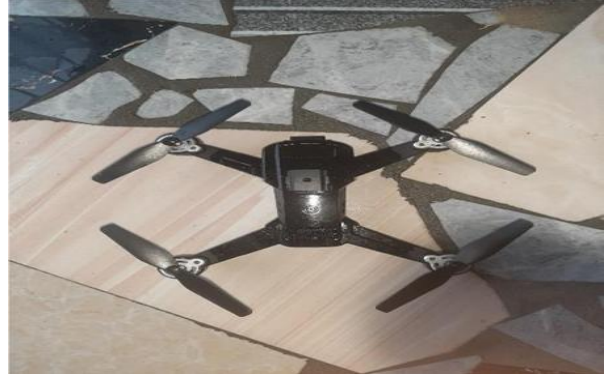
Figure 1: Constructed Quadcopter Drone with Camera
