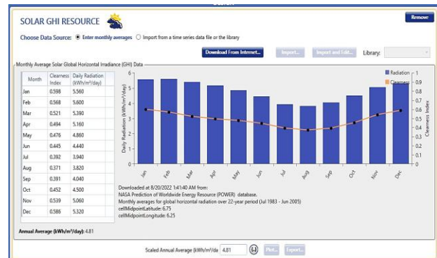
Figure 4.: Solar radiation data obtained from NASA by HOMER Pro software for a 22yrs period
